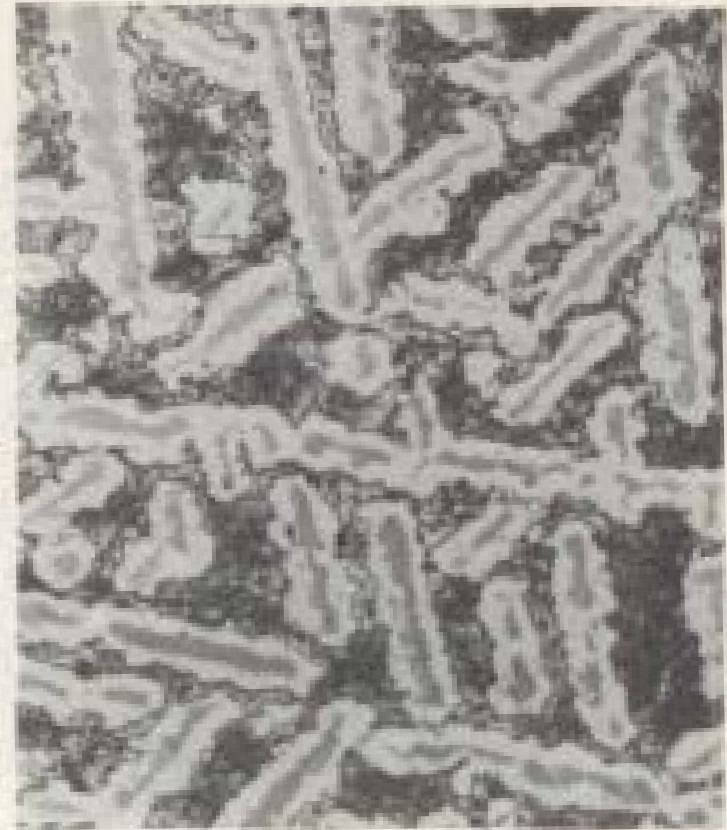
Figure 4.87 (a) Part of the copper-tin equilibrium diagram. (b) Microstructure of Sn-35 at % Cu alloy, showing primary crystals of \epsilon (grey phase) coated with \eta (white phase) in matrix of eutectic (mottled regions)
