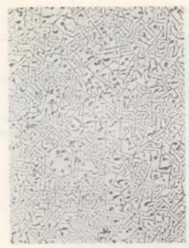
Figure 4.69 Transverse microstructure of Al–Si; grown at a very slow growth rate and in a steep temperature gradient ( \times 50 ) (Courtesy of M. G. Day 21 )
